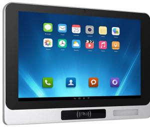
PC Industrial Touchscreen Capacitivo de 10,1" e 11,6" com processador Realtek RK3568 Cortex-A17 Quad Core 1.99GHz, 4GB RAM, 32G EMMC, compatível com Android 12.
